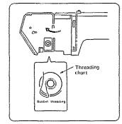
Bobbin threading chart is located behind the face cover plate.
